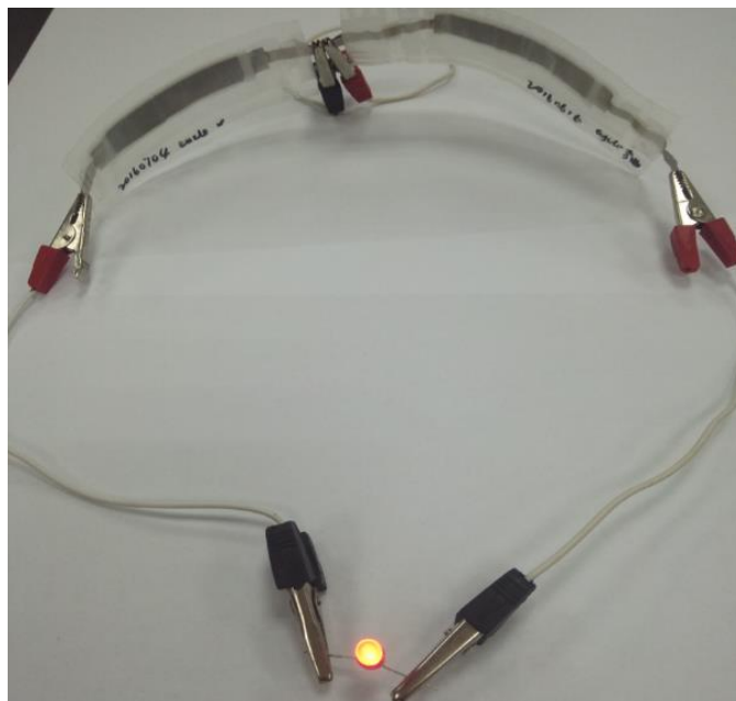
Figure S11. A red light-emitting diode (LED) powered by two flexible belt-shaped \text{Na}_{0.44}\text{MnO}_2//\text{NaTi}_2(\text{PO}_4)_3@\text{C} SIBs connected in series.
