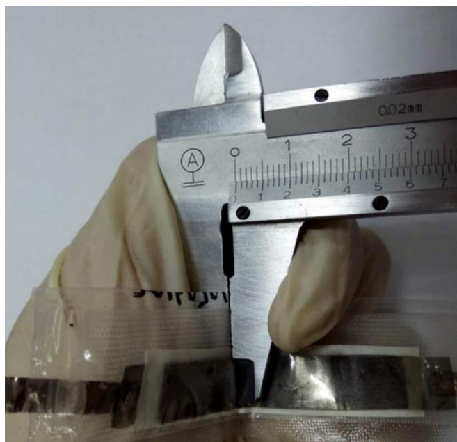
Figure S10. Photo profile of thickness measurement of the flexible belt-shaped \text{Na}_{0.44}\text{MnO}_2/\text{NaTi}_2(\text{PO}_4)_3@\text{C} SIB using 1 M \text{Na}_2\text{SO}_4 as electrolyte.
